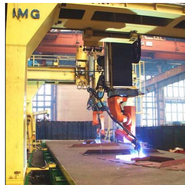
Welding Robot at work using IMG technology. Micro Panel Line, Aker MTW GmbH Germany
