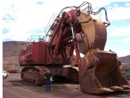
Andy inspecting the wear components on the O&K RH200 hydraulic face shovel used for the mining of iron ore.
