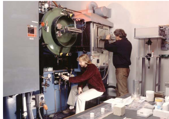
ANSTO's laser dilatometer system
