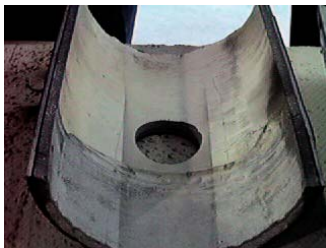
Abrasive water jet cut hole in concrete-lined steel water pipe
