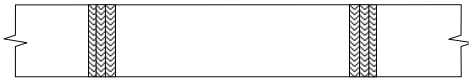
Figure 2. Top view of the rail head showing three transverse runs at the run-out of the depression.
