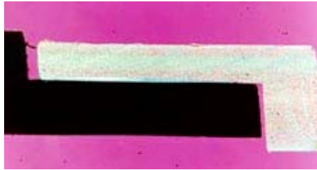
Figure 2: Transmission laser weld of clear to carbon loaded opaque material (Reproduced by permission TWI Ltd)
