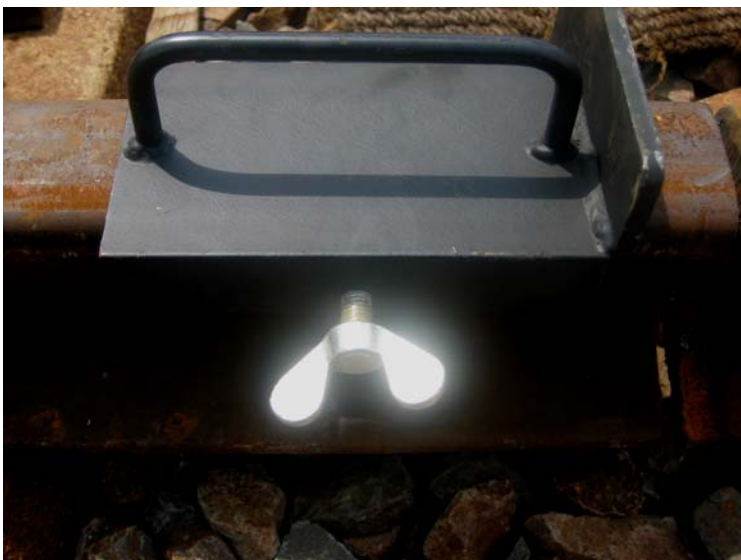
Figure 1. Example of cutting guide with handle and locking screw fitted on rail
